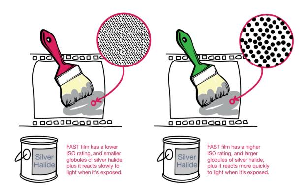
The larger the crystals, the more light sensitive they are and the smaller the crystals the less light sensitive they are. Once the shutter is open, the film reacts to the light hitting on it more quickly with larger crystals due to higher sensitivity. This is described as a higher or faster rating film. If you are using a lower rating or less sensitive film it will react less quickly to the light hitting it.
